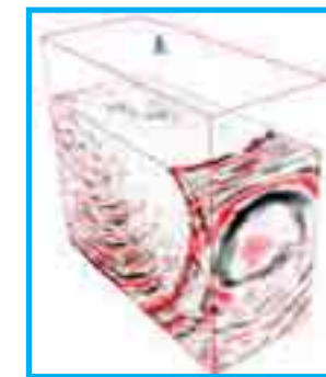
3C-3D Vector Migration of 3D VSP using S-Wave (salt flank) and P-Wave (sediments). Courtesy of OPEX.
